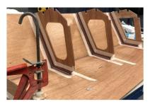
The bulkheads located and fitted
