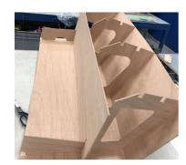
Dry assembly' of the Miracle section
